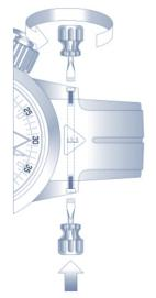
To dismantle the strap or the bracelet, the screws ® must be removed with a suitable tool or with two screwdrivers. In this case, the first screwdriver must be held in a vice, which serves as a holding device for one of the screws while the second one is used to unscrew the opposite screw in counter-clockwise direction
