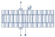
In order to close the lengthening system, fold up the extension links  $\bigcirc$  and return the central link  $\bigcirc$  to its original position by moving it downwards. Press down until the lock snaps in.
