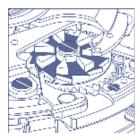
It is the sophisticated control centre which allows to start and stop the chronograph, and prevents the accidental setting to zero when the chronograph is working. Characteristics of this fine device are the remarkable technical value, the accuracy and the softness of its functions. Its realisation involves a total technical mastery both during the components production and the control and assembly phases.
